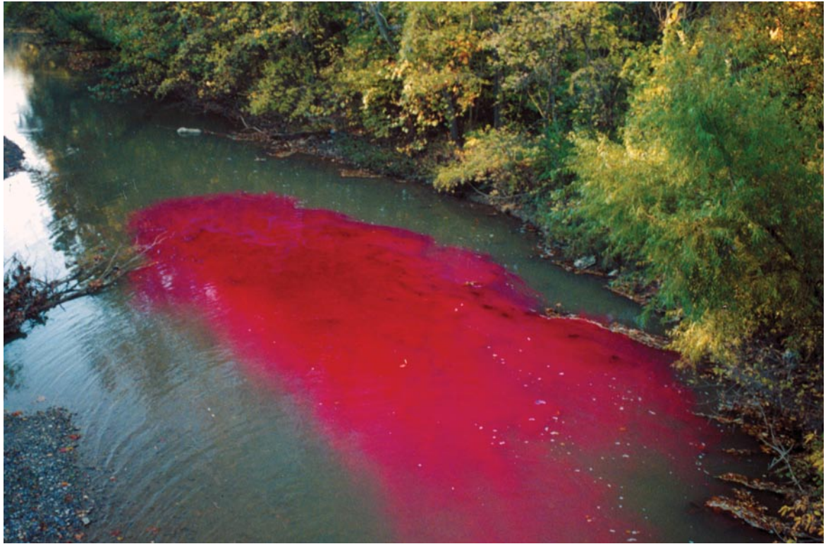
A plume of Rhodamine WT dye is seen shortly after being released in a river for a time-of-travel study.
